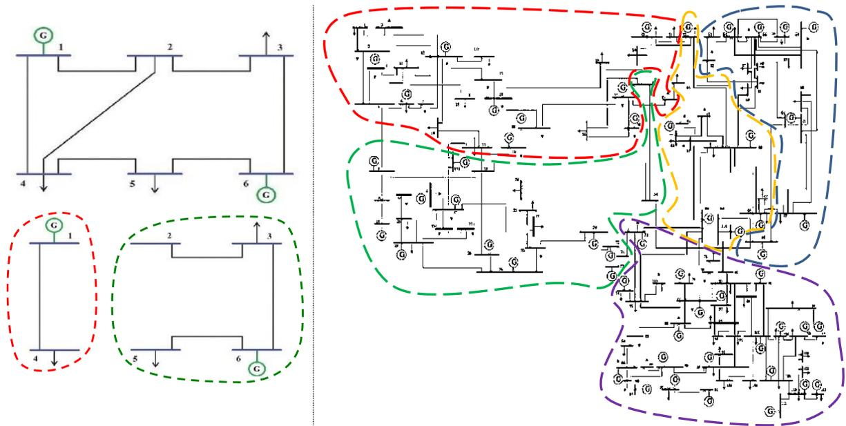
Figure 1: 6-bus IEEE test system before/ after sectionalization and 118-bus IEEE test system after sectionalization
