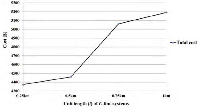
**Fig. 9.** Cost analysis for the DABS-E: total cost versus unit length of  $E$ -line systems
