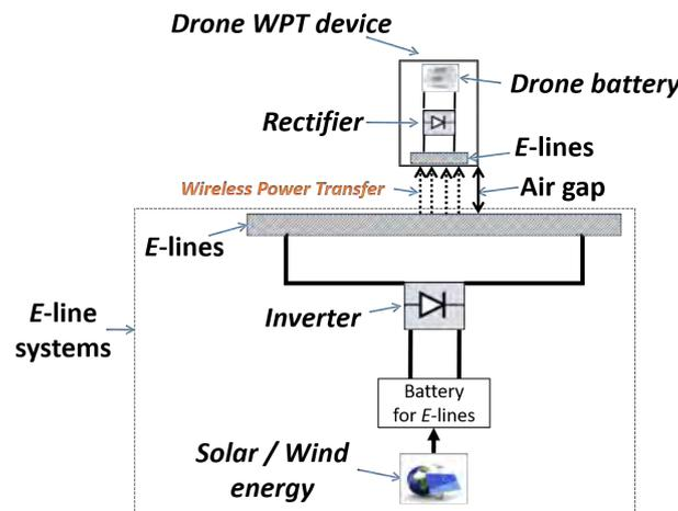
Fig. 2. Design of *E*-line systems
