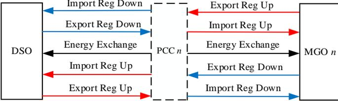
Fig. 2. Bidirectional energy and regulation exchange via the PCC
