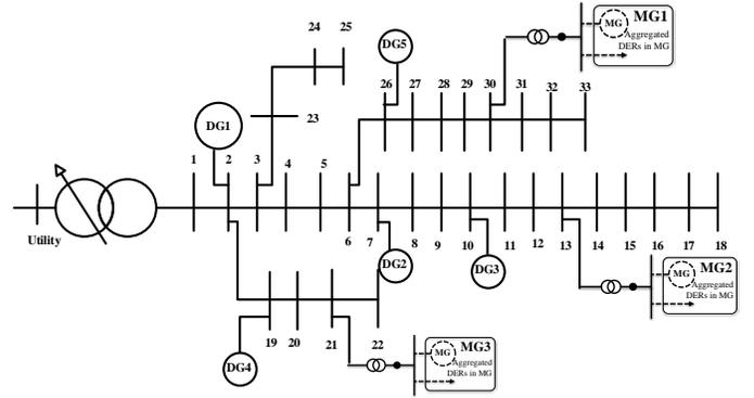
Fig. 4. The modified IEEE 33-bus distribution system
