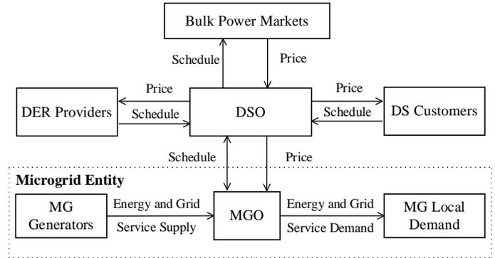
Fig. 1. A joint transactive distribution electricity market structure
