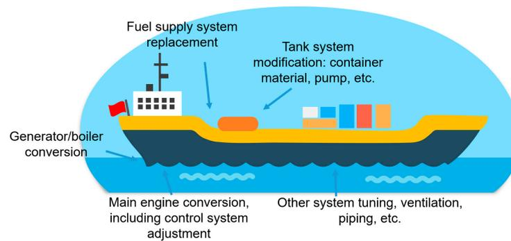
**Figure 1.** Representative key retrofitting considerations for a ship to be “alternative fuel-ready”: modifications are necessary for the fuel tanks, main engine, generator/boiler, fuel supply system, and other system components.
